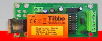
The interface module RS-LAN is an optional device for network communication of the fire control panels, manufactured by UniPOS with a personal computer through Ethernet network (LAN or internet).
